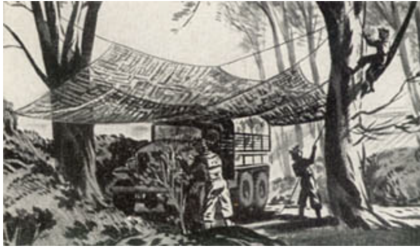
FIGURE 47 (1). An overhead screen provides good concealment. It is particularly valuable over more permanent parking places because it allows considerable freedom of movement underneath it and because vehicles can come and go while the camouflage remains in place. With this type of cover, a tight flat screen is unnecessary.
